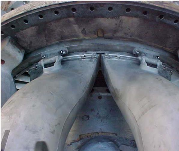
*Transitions bolted into place and locked*
